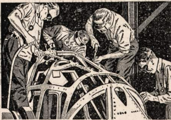
At Willow Run the top section of the bomber's enclosure, formerly made in 13 hand-formed pieces—is now made in only 3 parts—saving 30 hours in the construction time of each bomber.
