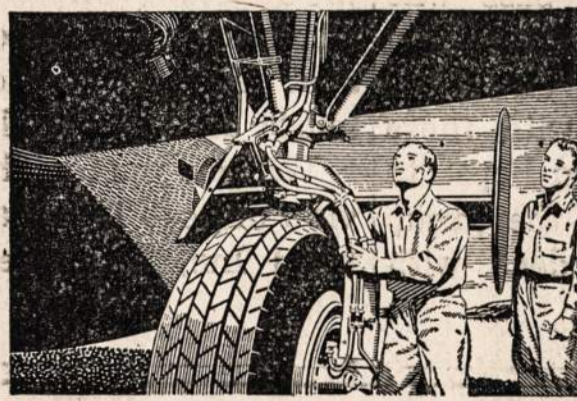
The airplane landing gear hinge formerly made of nine hand-welded parts, is now cast in one piece, eliminating 90% of the tools formerly used. Thus again Ford methods save time and materials.
