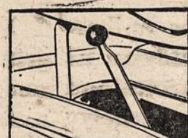
Shifting Lever—Forward, Neutral, Reverse
